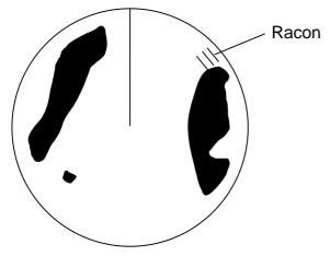
Figure 3-9 Appearance of racon signal on the display
